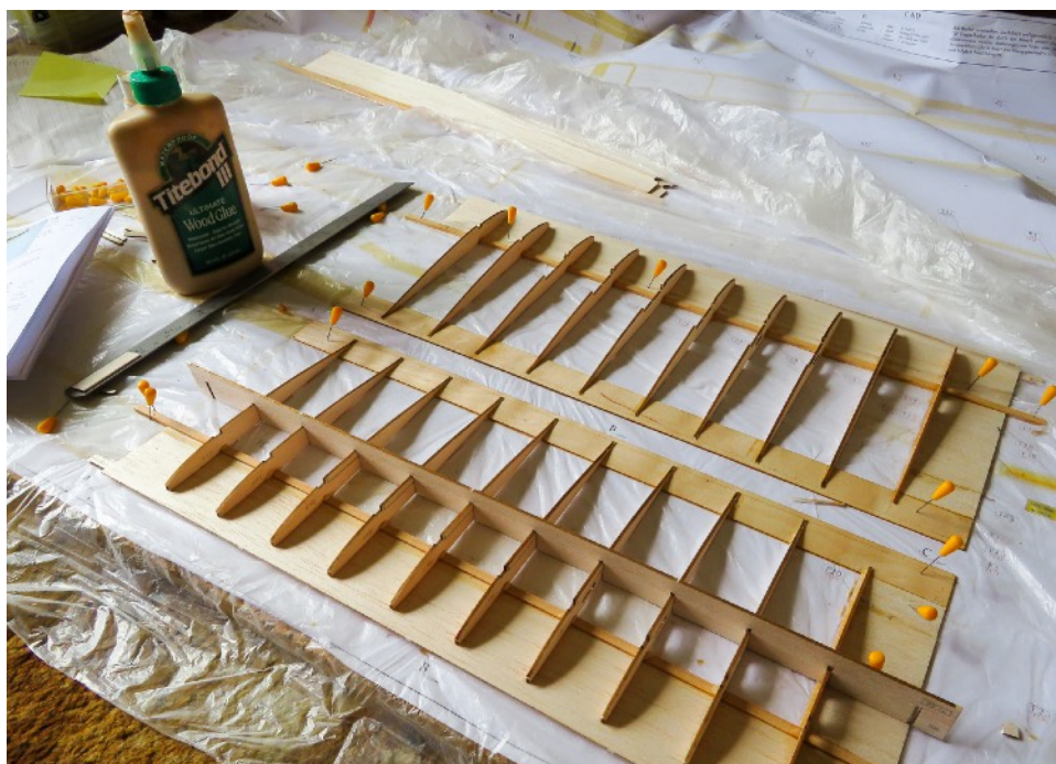
Wing panels under construction, note jig in use.
